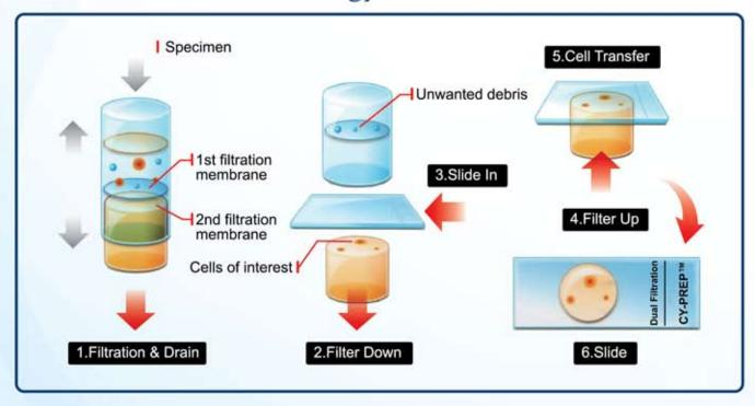
NOW, with the CY-PREP™ dual filtration technology, unwanted debris are effectively removed at the 1st filtration membrane, leaving only the wanted cell materials for investigation to be captured at the 2nd filtration membrane for transfer onto the glass slide.
