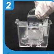
Insert reagent container into reaction cartridge.
