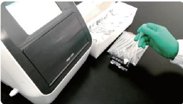
2. Pipette 800 ul urine sample to the sample loading chamber of the kit
