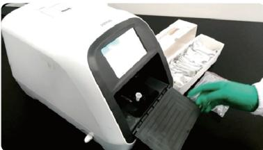
3. Place the kit loaded with samples in the instrument, note it should be placed horizontally, then cap it
