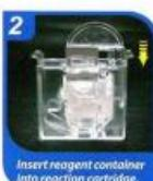
2 Insert reagent container into reaction cartridge.
